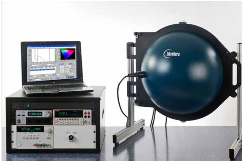
Figure 121. Labsphere’s TOCS system to measure IESNA LM-79 and LM-80 recommendations for LED characterization.
