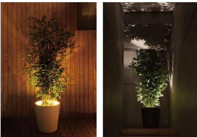
Figure 149. Scallops of light on a wall from nearby downlights and the shadows produced from an uplight under a plant or a small sculpture can create areas of visual interest that give character and individuality to a space.
