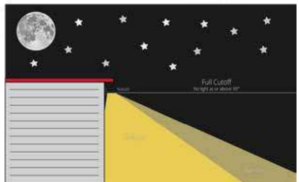
Figure 64. An illustration depicting the light spread of a full-cut off wall pack light
